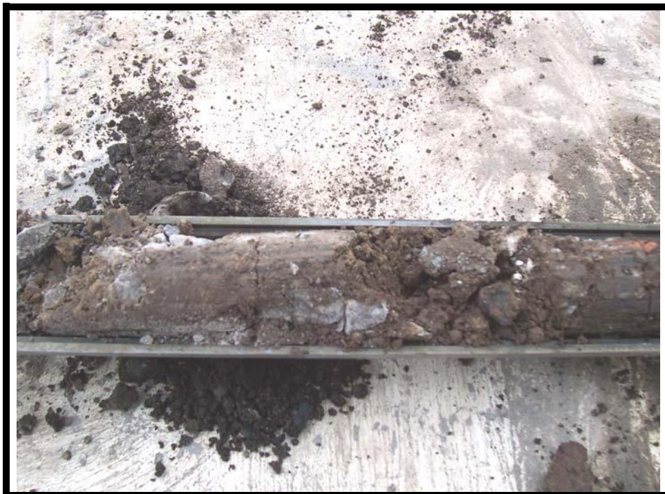
View of foundry sand with trace gray, white, black metallic and blue-green slag encountered in fill material collected from boring BS-39 [4.0' to 5.7'].
