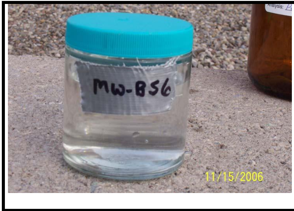
View of the purge water from well MW-BS6 at the time of sampling.
