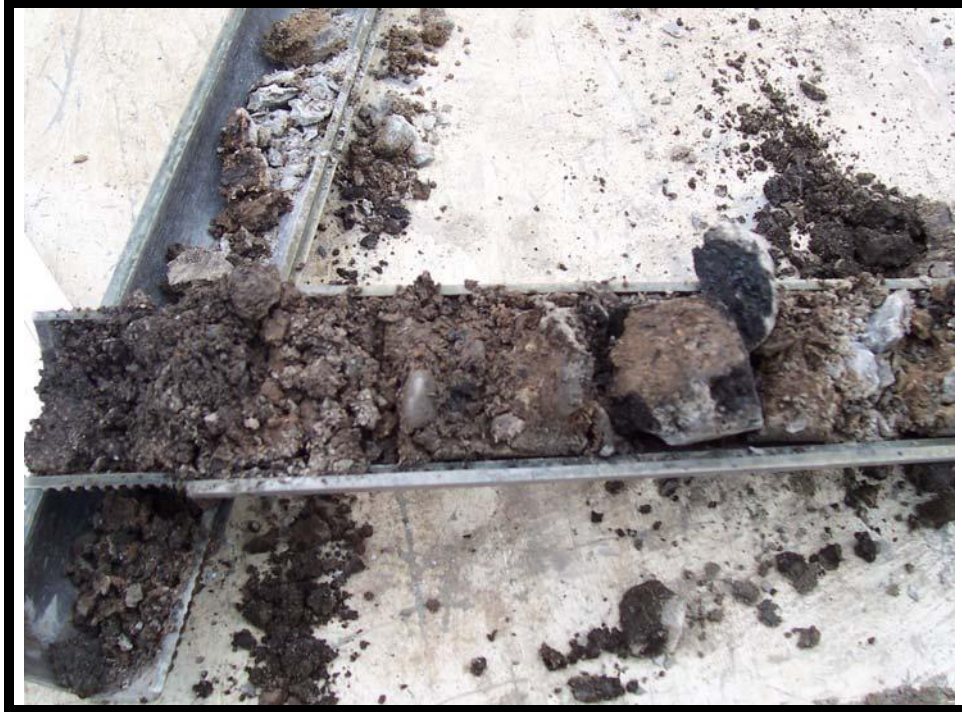
View of foundry sand and gray and black metallic slag encountered in fill material collected from soil boring BS-27 [4.0' to 5.5'].
