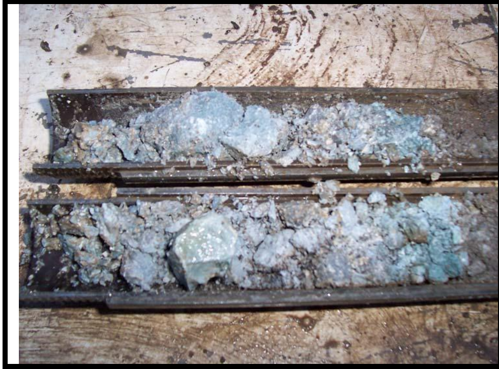
View of blue-green slag collected from boring BS-21 [4.0' to 4.5'].
