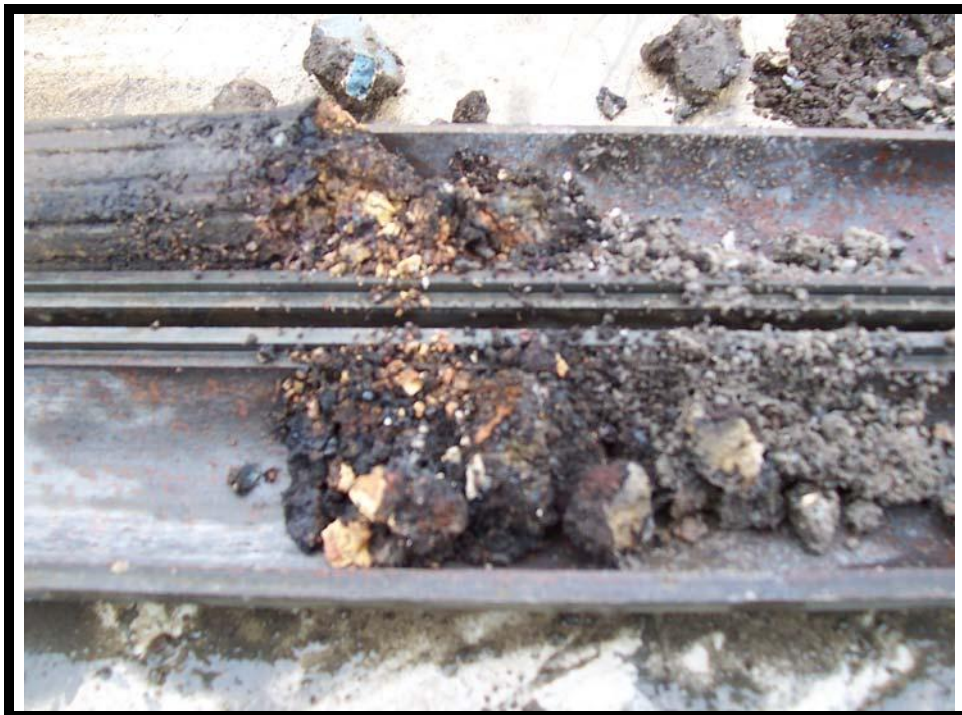
View of ash, cinders and black metallic slag encountered in fill material collected from boring BS-25 [2.0' to 3.2'].
