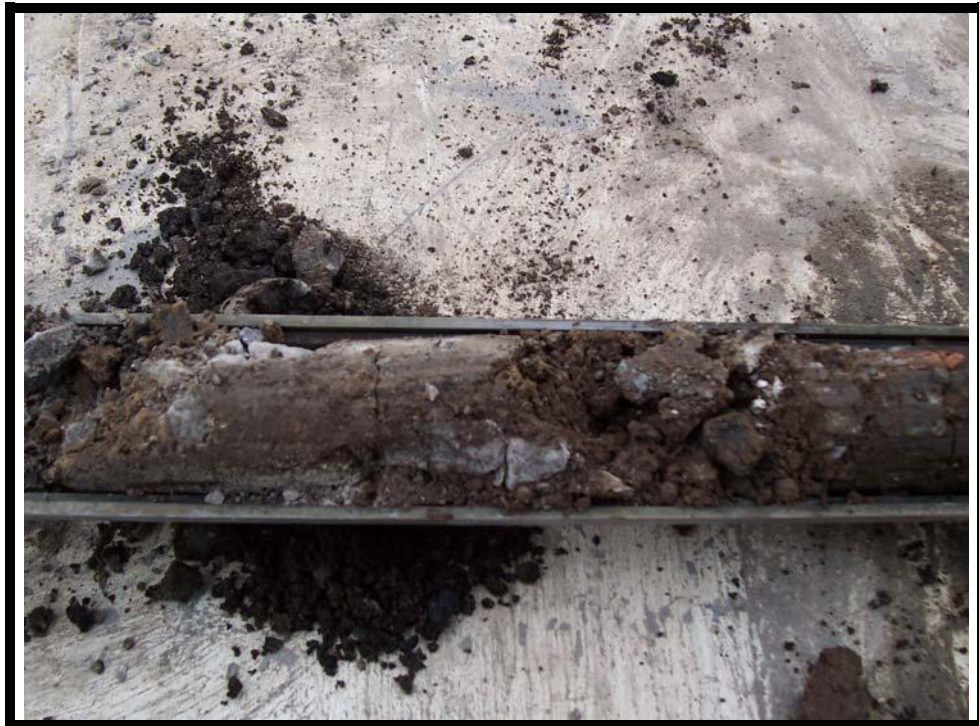
View of gray and blue-green slag collected from soil boring BS-20 [0.0' to 1.5'].
